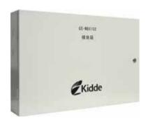
The GS-MBX102 module box is for in-door use, with enclosure protection class IP30. Used mainly for centralized installation and protection, it can accommodate 20 small modules or 12 large modules.
