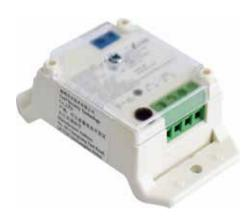
The GS-MOD8043 input module is mainly used to connect the equipment which provides normally open or normally close dry contact output signal, such as a flow switch, pressure switch, or butterfly valve. Once the module detects the action of the equipment, it will send the signal to fire alarm control panel.
