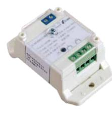
The GS-MOD8032 isolator module is mainly used to isolate the shorted circuit of the branch bus from the complete loop to ensure normal operation of other parts and locate the isolated part. Once the short circuits faults been fixed, the isolator module will auto restore this part to the normal loop.
