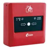
J-SAP-M-GS8030 is an intelligent manual call point for indoor use installed in public places. With the manual confirmation of a fire, press the button on the call point to send an alarm signal to the fire alarm control panel, then the panel will display the location, address, etc. information of the call point, meanwhile triggering the alarm sound. Once you plug in the handheld fire phone handset into the telephone jack on the call point, it will directly call the fire phone panel automatically.
