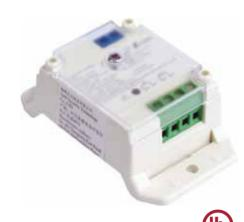
The GS-MOD8031 isolator module is mainly used to isolate the shorted circuit from the complete loop to ensure normal operation of other parts and locate the isolated part. Once the short circuits faults been fixed, the isolator module will auto restore this part to the normal loop.
