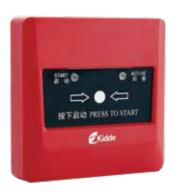
J-SAP-M-GS8030X is an intelligent hydrant call point with a high degree of protection. After pressing the button on the unit, the red START indicator will be on, means the alarm signal has been sent to the fire alarm control panel. Once the fire pumper is running, the unit will light the green ACTIVE indicator.
