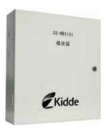
The GS-MBX101 module box is for in-door use, with enclosure protection class IP30. Used mainly for centralized installation and protection, it can accommodate 10 small modules or 6 large modules.
