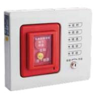
The GS8204 addressable manual/ auto switch is an important part of a gas release system as well. Under the manual mode, the gas will not be released even if the alarm has been triggered. Under the auto mode, the gas releasing will be based on the settings and programming. It will be set to manual mode when someone enters the protection area. GS8204 is an addressable device, direct connect to gas release control panel 2<sup>nd</sup> communication bus.
