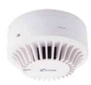
JTY-GDM-GS8010 intelligent photoelectric smoke detector is a point type device that can detect fire with infrared scattering technology. With the built in microprocessor and smoke detection algorithm, it can judge the fire condition and trigger the alarm by itself.
