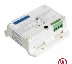
GS-MOD8041 input/ output module is mainly used to connect the equipment which needs to be controlled by fire alarm control panel, such as exhaust valve, fire damper, etc., it also can receive the action signal of the controlled equipment and send it to fire alarm control panel.
